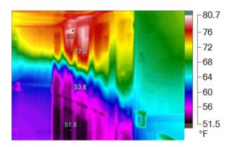
Even in a fully contained cold aisle, low raised-floor static pressure and open spaces in cabinets cause variances in intake temperatures. Conditioned air that reaches the aisle is lost through the open spaces in the racks. Servers pull exhaust air from the back of the racks through open spaces at the top. Sealing cable openings and installing blanking panels help improve cooling unit efficiency.
